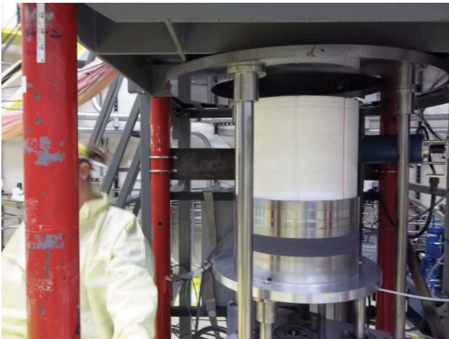
Fig. 8. BeO reflector (white) and bottom shield (silver and black) on Comet movable platen.
