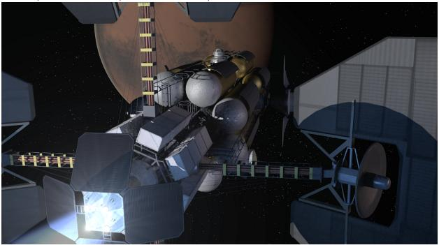
Rendering of a 40 MW VASIMR® Nuclear Electric Propulsion (NEP) human mission to Mars (Credit, Ad Astra Rocket Company)
